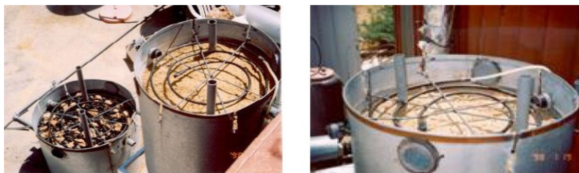
Figure 4.1: Distributing laterals with large pore size Figure 4.2: Biofilters with sand layer prior washout
